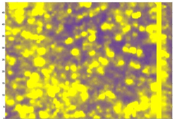
Steel slag, in its pure form has a very low electrical conductivity, in contrast to the flue dusts which have a high metal content and a correspondingly high conductivity. Skulls, being almost entirely ferrous metal have an extremely high conductivity, generating an even greater electrical contrast against slag. These observations led to the conclusion that electromagnetic methods would be
