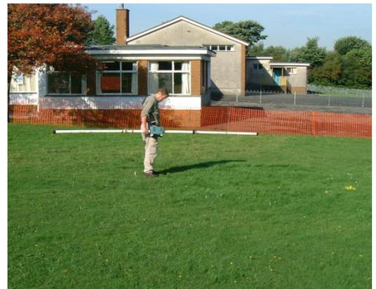
The slag landfill was known to have been a dumping ground for not only slag wastes but also fine flue dusts and large metallic lumps known as skulls. The piling contractor did not wish to hit obstructions and also needed to know where the piles would encounter fine dusts rather than slag. Geotechnology staff were invited to examine the site and the filling records to determine whether a geophysical method could be used to sense the presence of dusts and obstructions.
