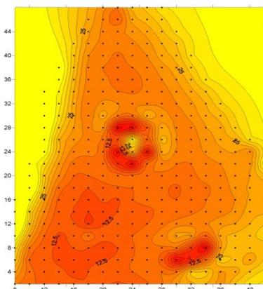
Other uses for EM include the assessment of contaminated land, as shown on the third image on this page. An EM61 survey taking one day to complete has sensed the presence of a gasworks tar pit (square), a liquor storage tank and even the buried pipeline connecting the two.
